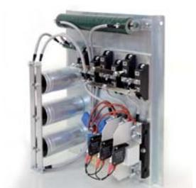
This type of special assembly is mainly used to protect power converters against overvoltages. Sudden current variations at system and commutating inductances may produce overvoltages which impose a load on thyristors or semiconductors in the reverse or blocking direction. Overvoltages may for example occur during the cutting out of semiconductors, the cutting in and out of power transformers, switching operations to inductive and capacitive loads,
