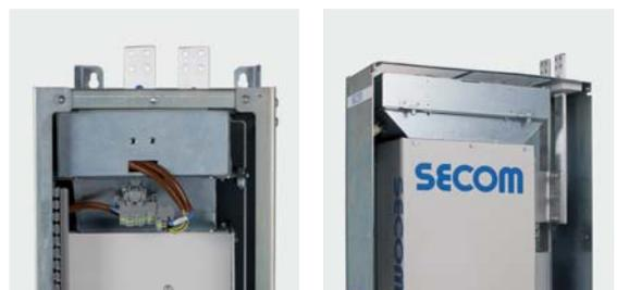
The GR9 converter is available in different configurations, with current range between 250 Amps and 1500 Amps and supply voltage range between 380 VAC and 850 VAC. Is an air cooled solution and all frames are equipped with internal fuses and thyristor snubber. As standard is supplied with IP20 protection degree (IP00 only by request).
